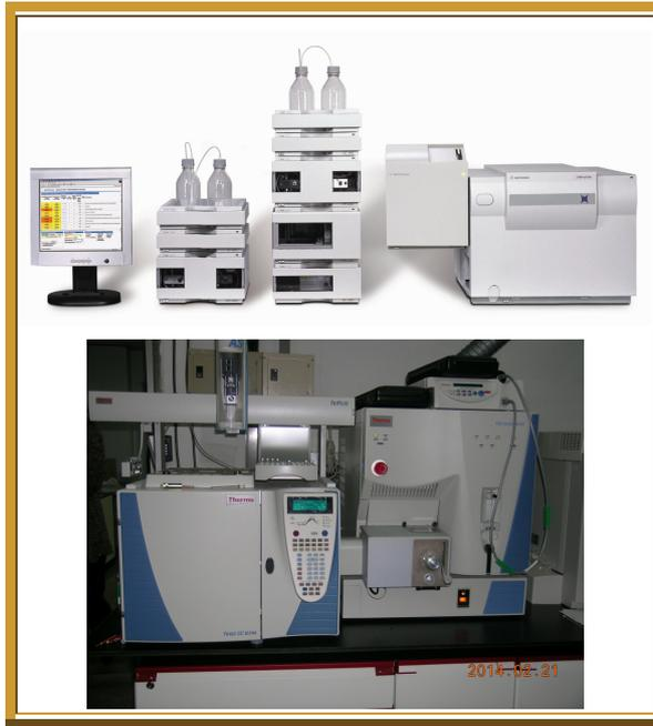
**LC/Ion-Trap MS and GC/MS/MS**
