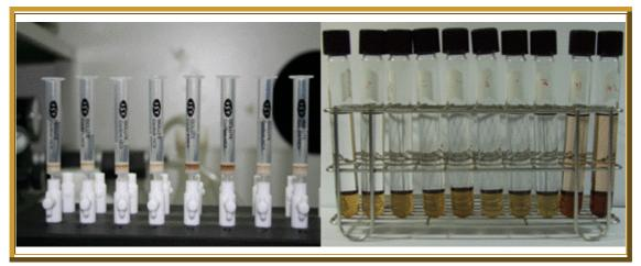
Solid phase extraction and liquid-liquid extraction for hair analysis
