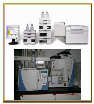
LC/Ion-Trap MS and GC/MS/MS
