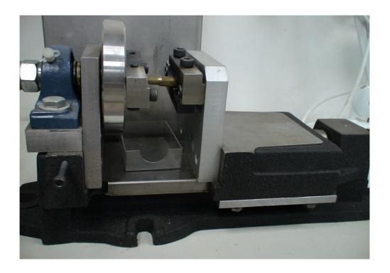
Instrument: Bullet disassemble instrument
