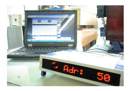
Instrument: Ballistic speed measurement system
